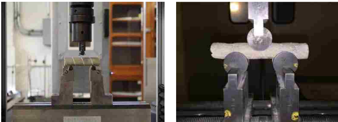
Figure 5.40. The setups of the SBS test in this research (left) and report of UM (right)
