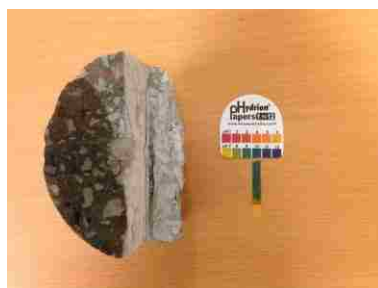
pH measurements using Grubb's method (left) and ASTM F710 (right) (Walker Bridge)
