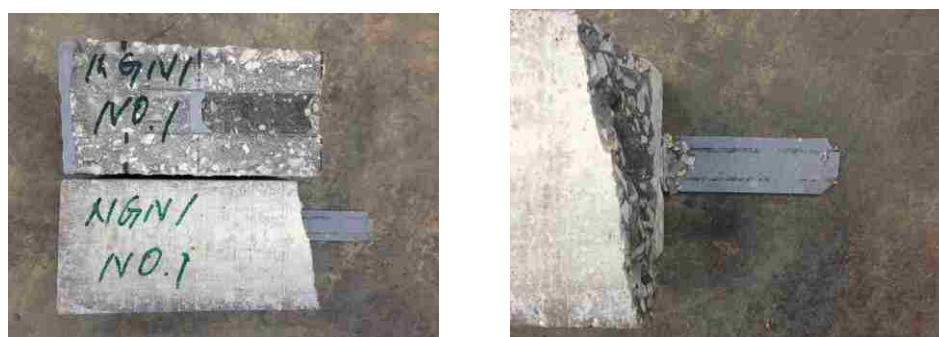
Figure 4.43. A representative failed specimen reinforced with micro-fine brass coating steel fibers under tap water (3,000 hours)
