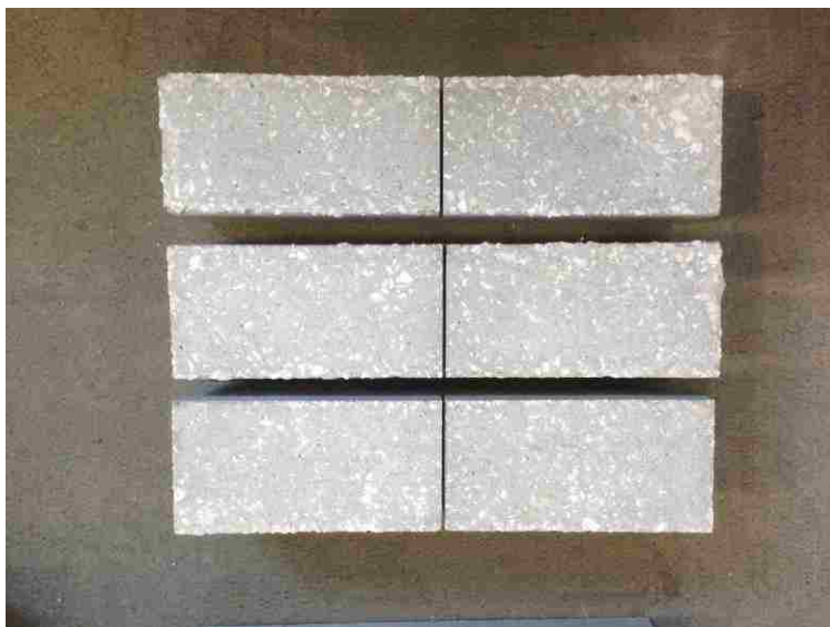
Figure 4.4. The specimens ground with the saw-cuts
