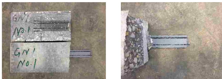
Figure 4.42. A typical failed specimen reinforced with galvanized coating steel fibers under tap water (3,000 hours)
