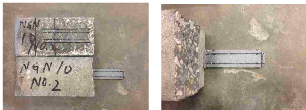
Figure 4.72. A representative failed RNG specimen under salt water (4,000 hours)
