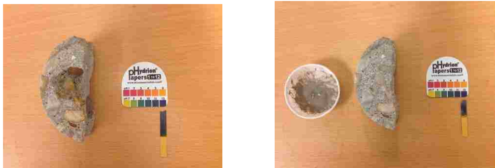
Figure 5.68. pH measurement of sample 1 (Southview Bridge): ASTM F710 (left) and Grubb's method (right)
