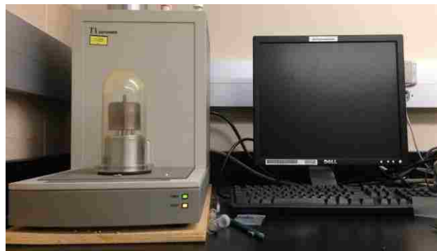
Figure 5.51. TA instrument for T_g measurement
