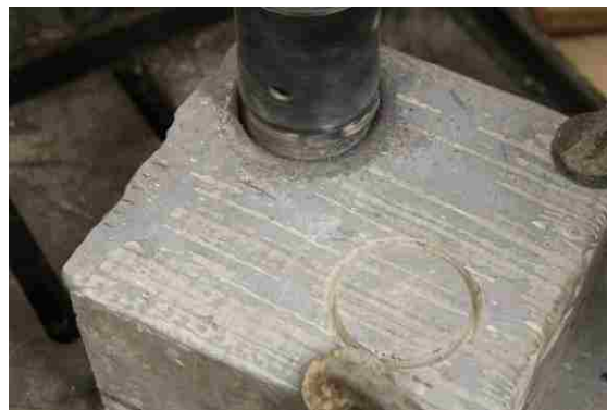
Figure 4.8. The detailed process of drilling core
