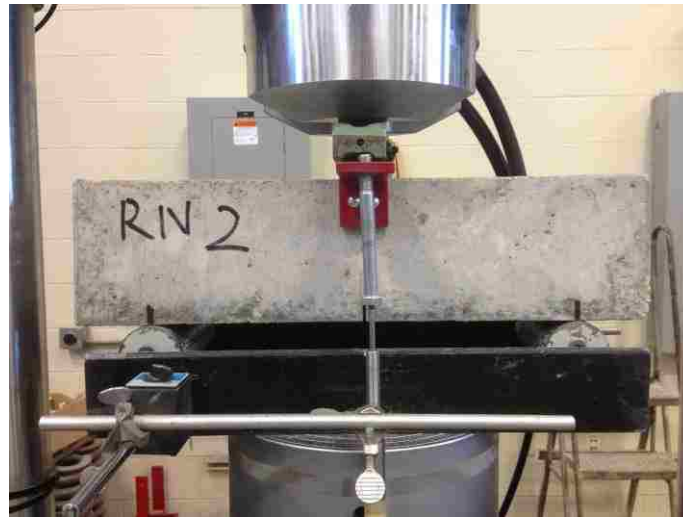
Figure 4.55. A typical three-point loading test configuration
