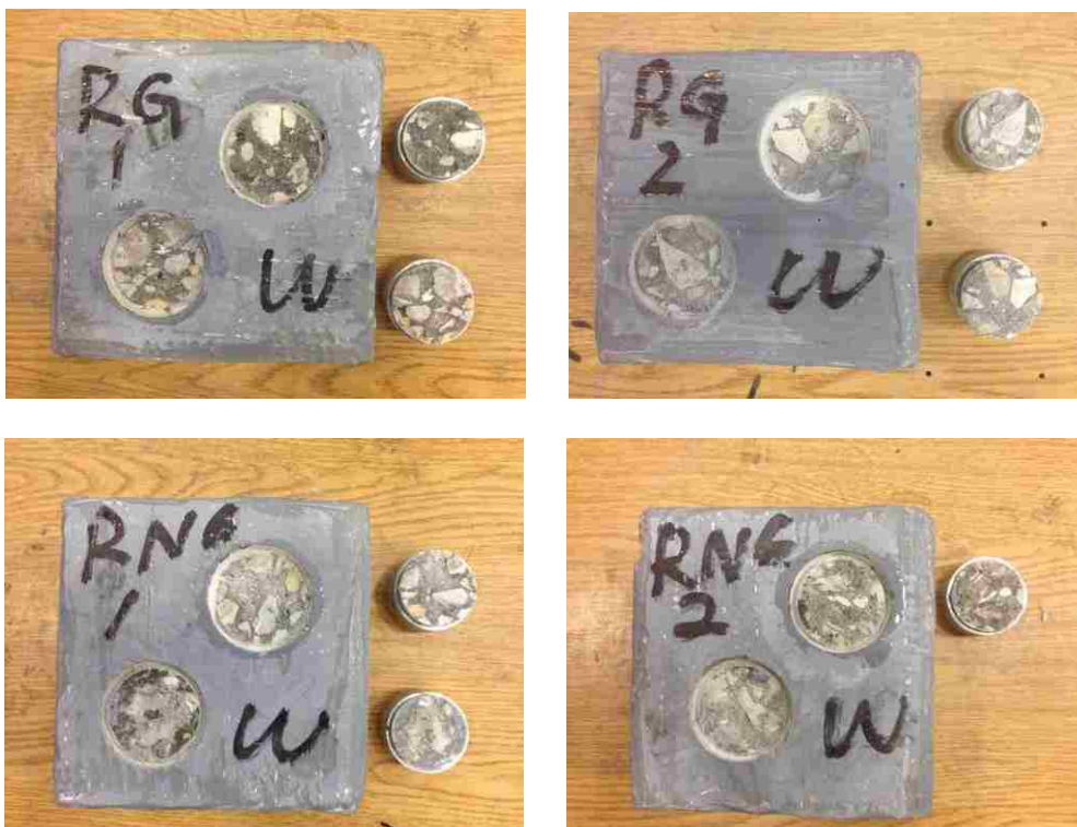
Pull-off RG and RNG specimens (water)
