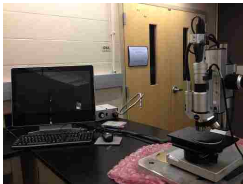
Figure 3.15. HIROX KH-87 Digital Microscope
