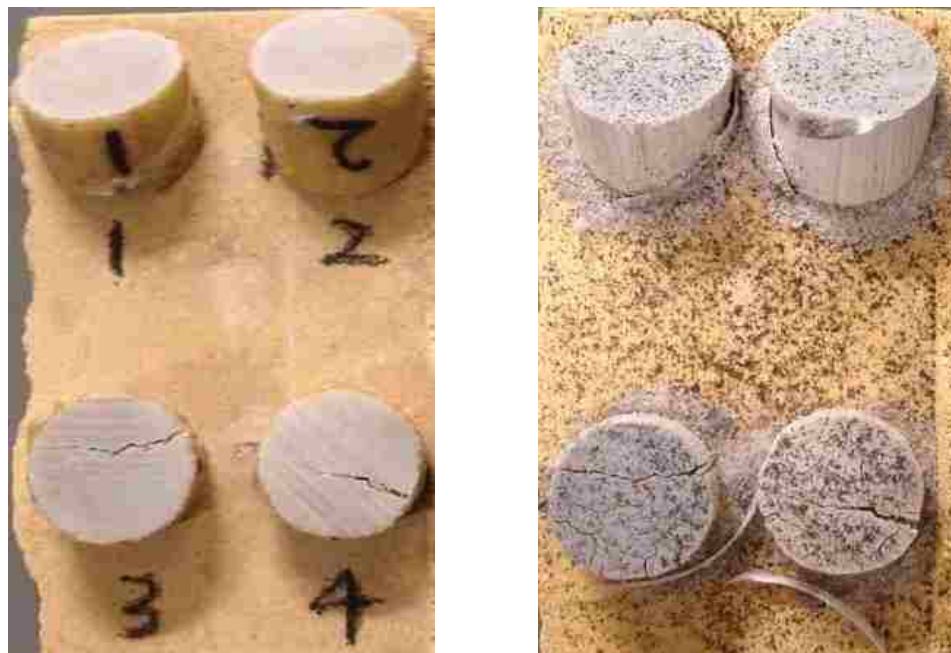
Figure 5.49. The #6 samples of before (left) and after (right) test for Sierrita de la Cruz Bridge
