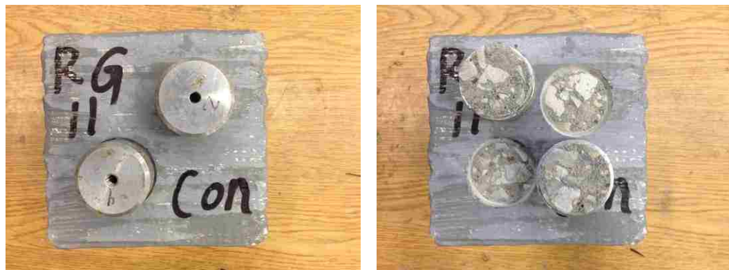
Figure 4.35. A typical control specimen with failure Mode G
