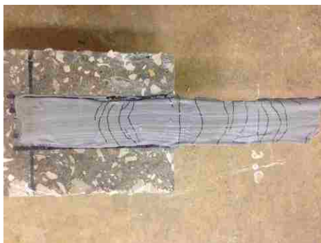
Figure 4.24. SRP sheet with curved lines in control specimen
