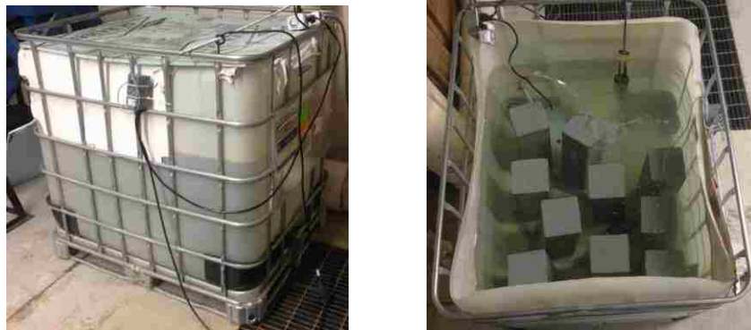
Figure 4.54. SRP specimens in hot water
