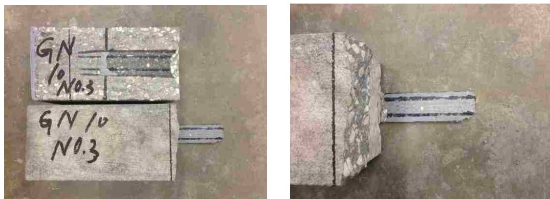
Figure 4.71. A typical failed RG specimen under salt water (4,000 hours)
