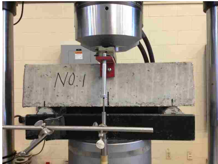
Figure 4.82. A typical three-point loading test configuration
