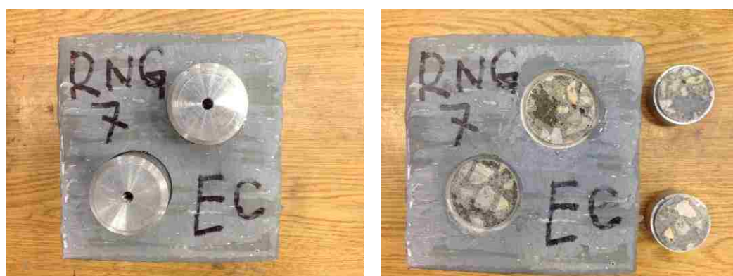
Figure 4.37. Pull-off specimens reinforced with brass coating steel fibers (Mode F)
