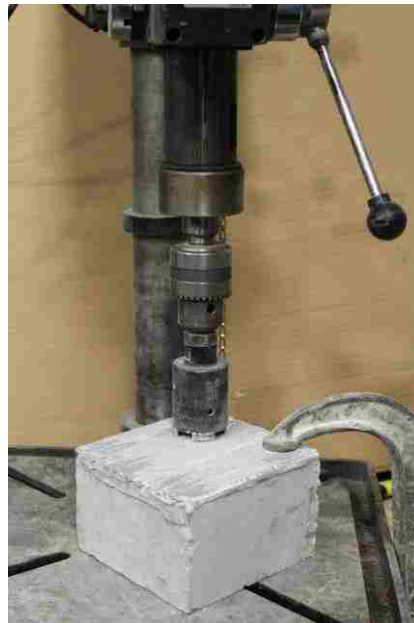
Figure 4.9. The process of drilling core
