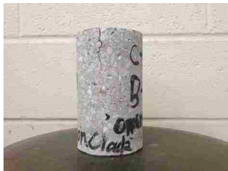
Figure 5.34. A representative concrete core with crack
