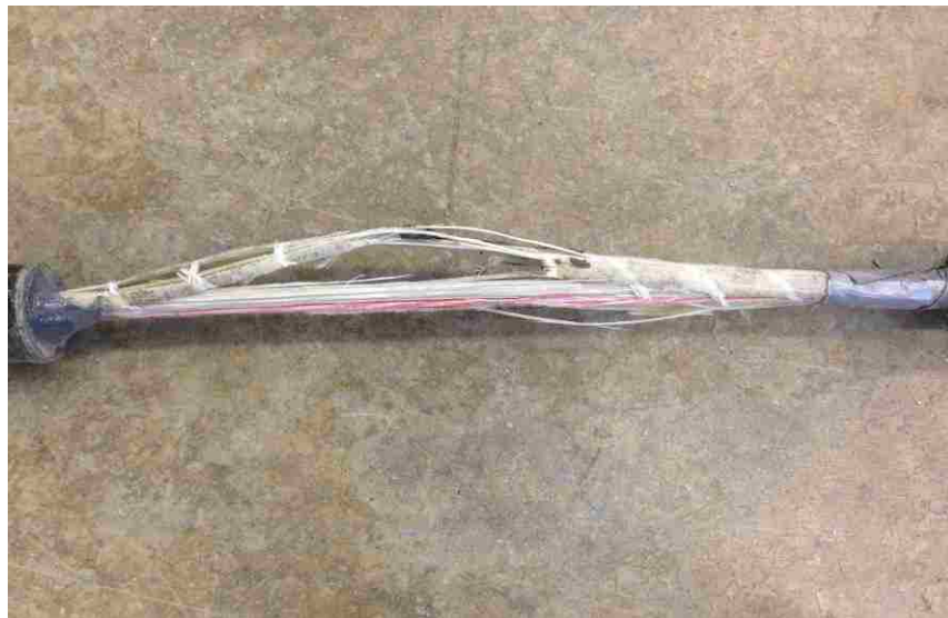
Figure 3.14. Typical failure mode of GFRP bar subjected to tensile test
