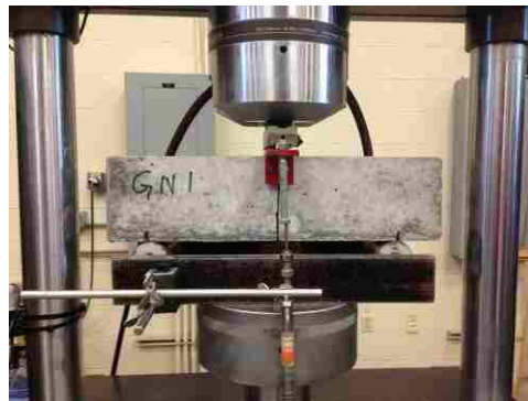
Figure 4.40. A typical flexural bending test configuration
