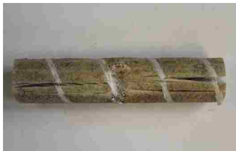
Figure 5.41. Failure #6 GFRP bar from Southview Bridge
