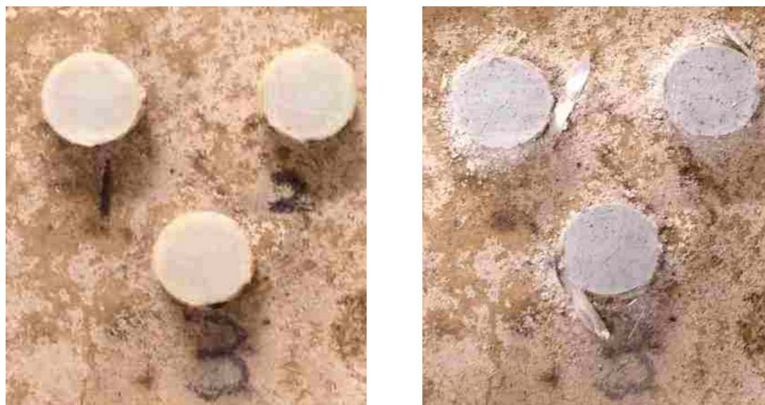
Figure 5.50. The #5 samples of before (left) and after (right) test for Sierrita de la Cruz Bridge
