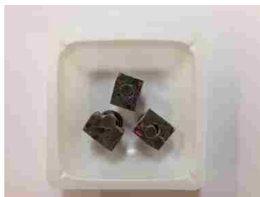
Figure 5.39. Prepared GFRP samples from core C-1 B-3 and core C-2 B-3 of Walker Bridge
