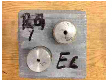
Figure 4.12. A typical pull-off specimen
