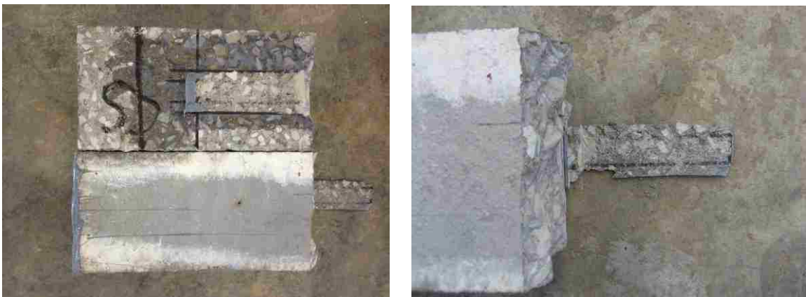
Figure 4.29. The failure mode of a typical control specimen reinforced with brass coating steel fibers (RNG 6, Failure Mode 1)
