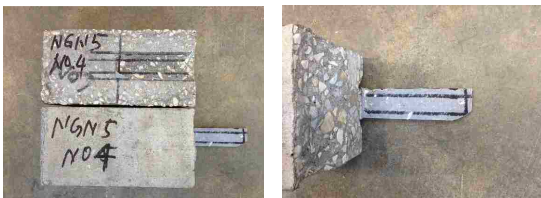
Figure 4.70. A failed RNG specimen under salt water (1,500 hours) (Mode 2)
