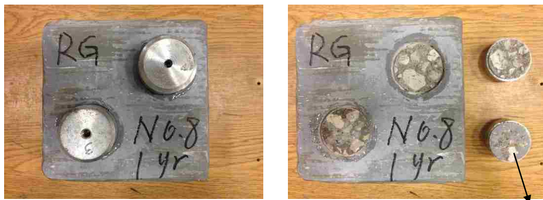
Figure 4.90. Pull-off RG specimen under the real-time weather and solar exposure
