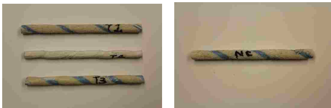
Figure 5.37. The extracted GFRP samples from core C-1 B-3 (left) and core C-2 B-3 (right) of Walker Bridge
