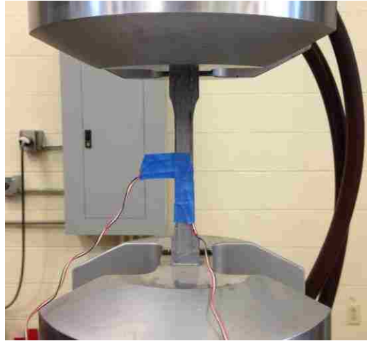
Figure 4.95. The setup of tensile coupon test
