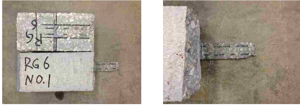
Figure 4.44. A typical failed control specimen (4,000 hours)
