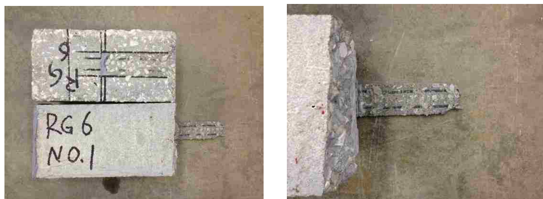
Figure 4.73. A failed control RG specimen (4,000 hours)
