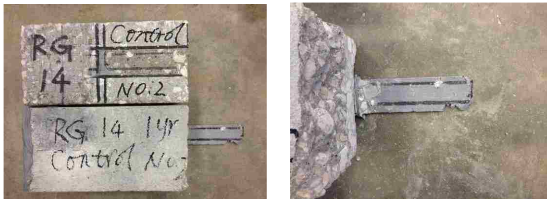
Figure 4.87. A representative failed control RG specimen reinforced
