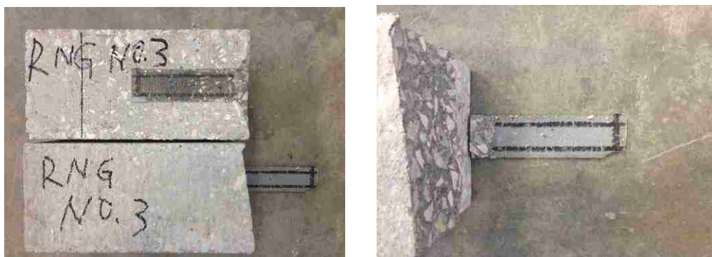
Figure 4.85. A representative failed RNG specimen reinforced (unloaded) exposed to field environment
