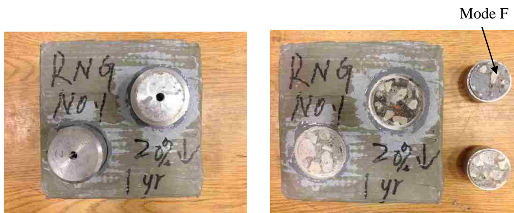
Figure 4.91. Pull-off RNG specimen under the real-time weather and solar exposure
