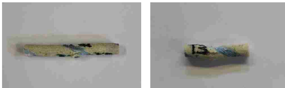
Figure 5.43. Failure T1 (left) and T3 (right) GFRP bars from C-1 B-3 of Walker Bridge
