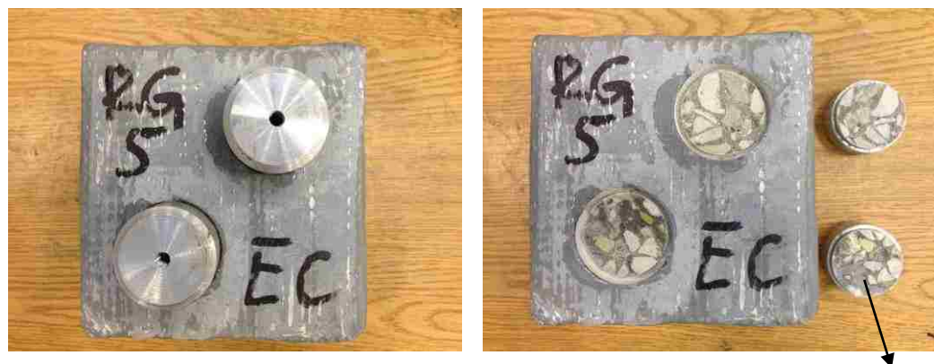
Figure 4.36. Pull-off specimens reinforced with galvanized coating steel fibers (Mode F)
