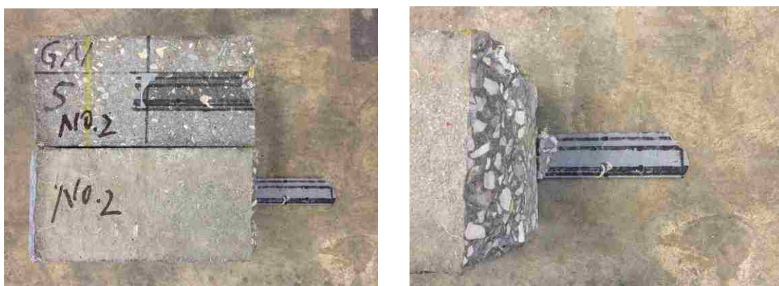
Figure 4.69. A typical failed RG specimen under salt water (1,500 hours)
