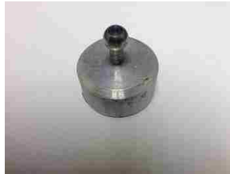
Figure 4.11. A typical dolly with a pull pin
