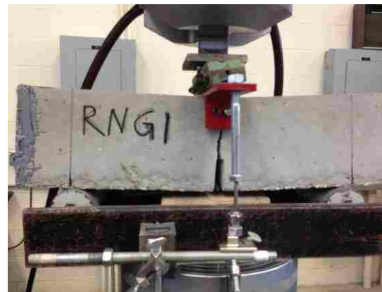
Figure 4.21. A typical failed SRP specimen
