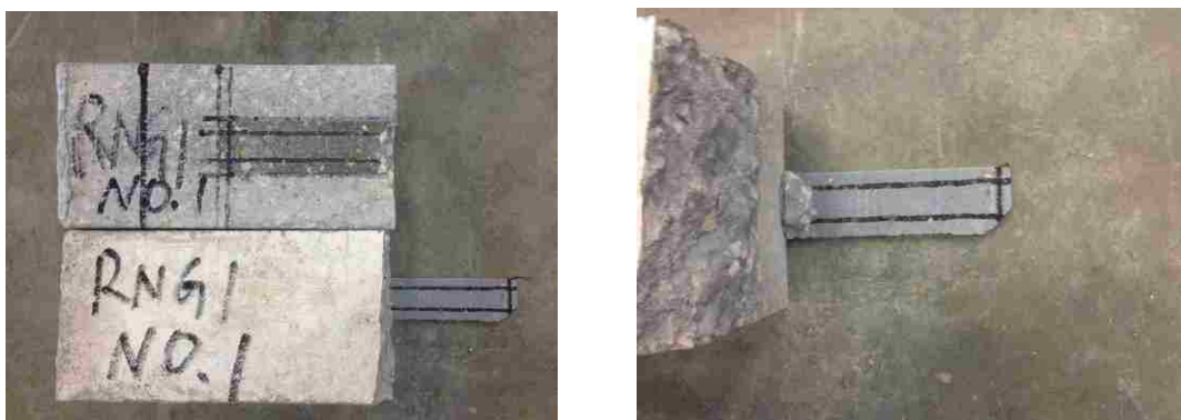
Figure 4.58. Failed RNG 1 (4,000 hours)
